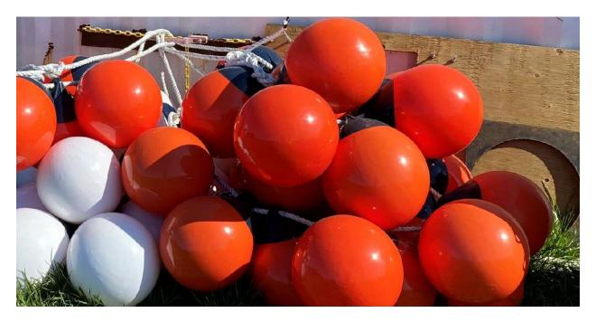
The <u>white round</u> buoys will identify anchors that Dredge America has placed in the lake either to hold the pipeline in place or for the dredge to swing from. These buoys should always be floating.
